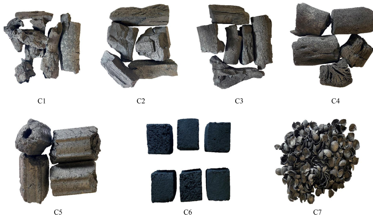
Fig. 1. Photographs of the different charcoal types. C1: Oak wood charcoal, C2: Orange wood charcoal, C3: Valonia oak wood charcoal, C4: Marabu wood charcoal, C5: Extruded charcoal from beech wood, C6: Coconut shell charcoal, C7: Hazelnut shell charcoal.
